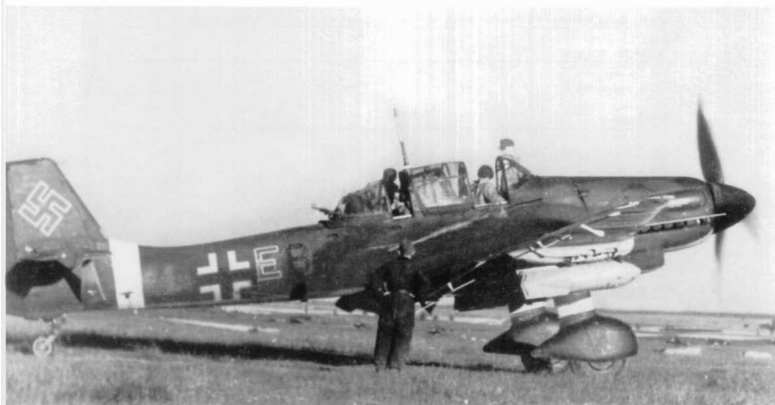
Probably also photographed in the summer of 1944 was this heavily-loaded Ju 87 D-5 of Stab I./SG 1. Just visible aft of the fuselage Balkenkreuz is an area where the original A5 lettering had been painted out and replaced by smaller lettering.
