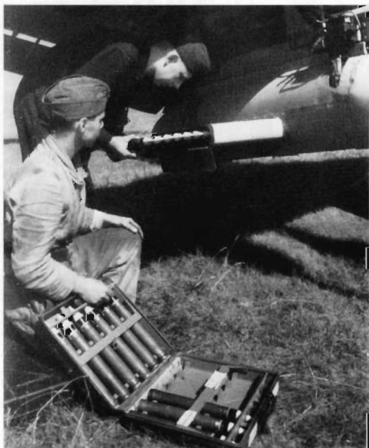
Two views of a Luftwaffe armourers about to load a clip of 37 mm anti-tank rounds into the magazine holder of a BK 3.7 cannon.
