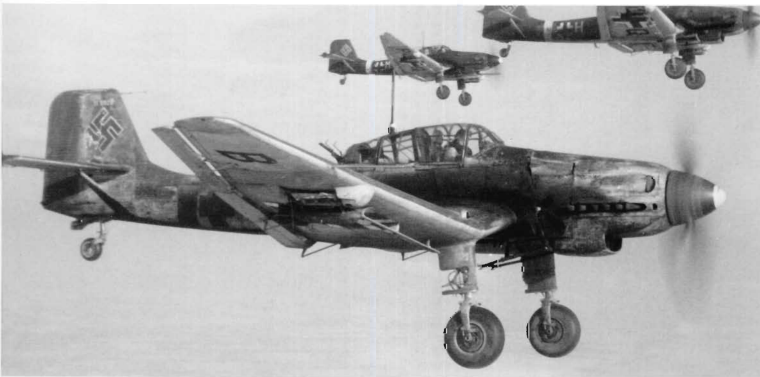
Above: Snow camouflaged Ju 87 D-3s of an unidentified unit in the winter of 1942/43. Note the towing attachment under the tail and the extent to which components have been removed from the undercarriage.
