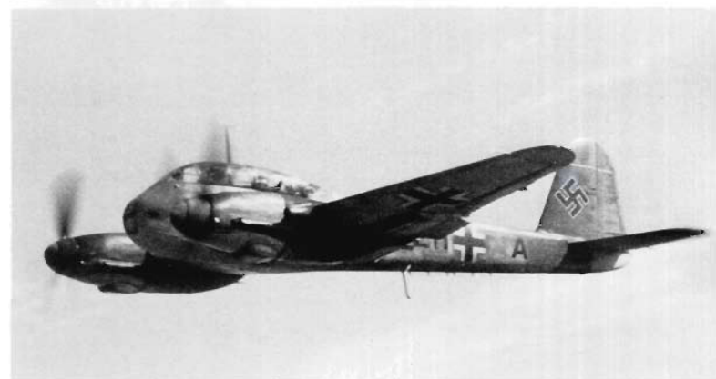
An Me 210 A-1 W.Nr. 2100182 belonging to Versuchstaffel 210 coded 2H+AA. From the outset it was intended to fit dive brakes as standard to the Me 210 although due to the poor handling of aircraft it was never used in the role of dive bomber. This machine was later transferred to III./ZG 1 and was destroyed by flak on 5 December 1942.
