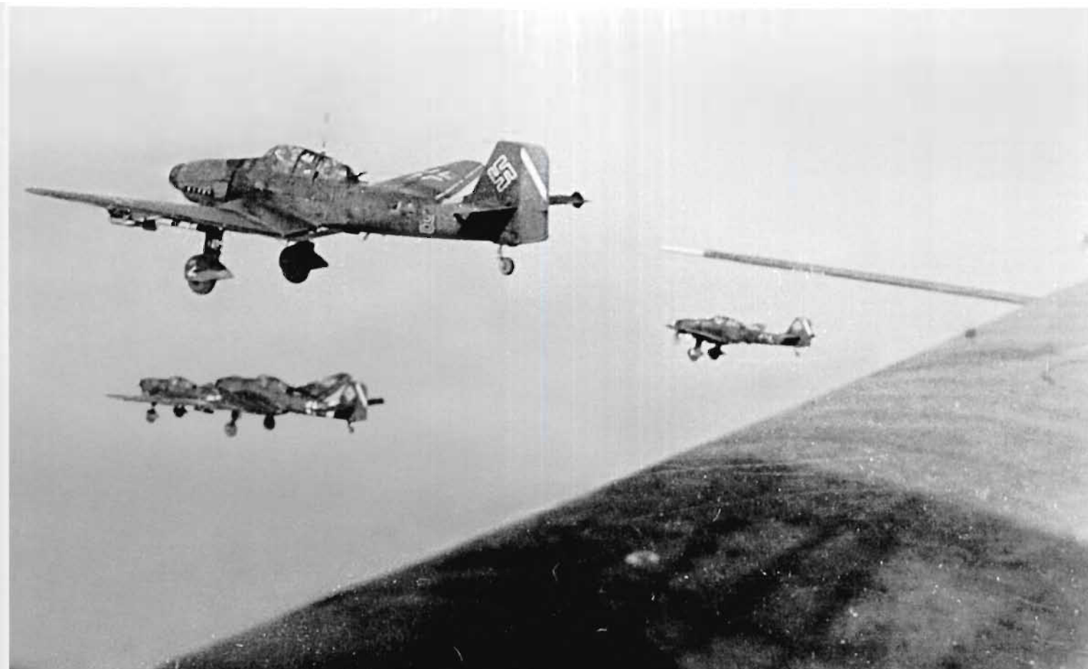
Two views of Ju 87 D-3s of 4./St.G 2 enroute to a target in Russia. The aircraft in both views T6+BM, which as a 'White 2' painted on its wheel spat has had its leather oleo shock-bands (compression cover) removed from the undercarriage fairings. The white stripe on the rudder was an additional Staffel identification.
