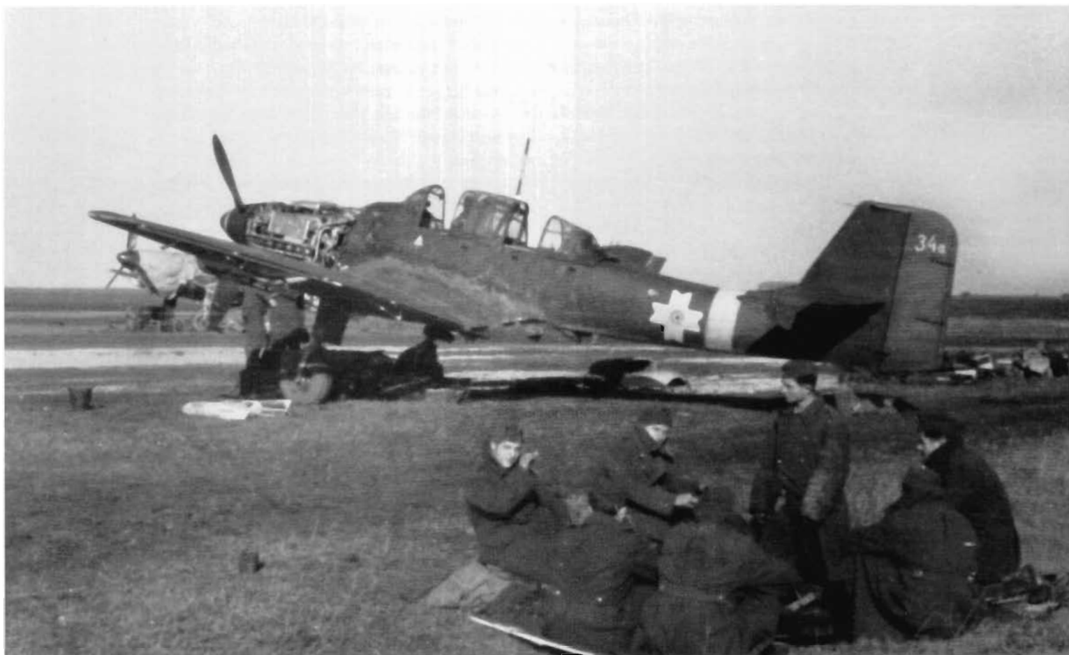
A Rumanian Ju 87 D-3 undergoing engine maintenance, probably in the early spring of 1944.
