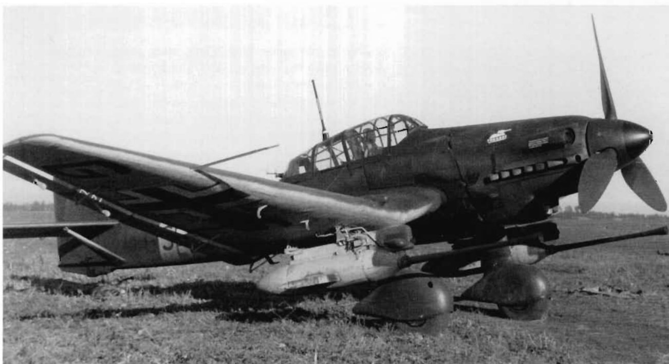
Two views of a Ju 87 G from St.G 1, marked with the T-34 Panzerknacker badge. The aircraft were often called Kannonenvogel (the "gun bird"). Thought devastating to Soviet armour these twin 37 mm cannon equipped Ju 87 Gs suffered a loss of speed and manoeuvrability due to the additional weight of the cannon at 700 kgs (350 kgs each).
