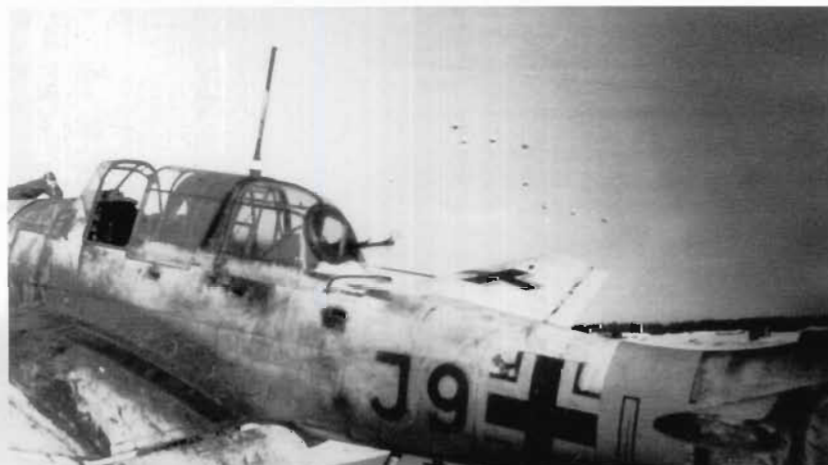
Left: The Staffel letter L on this Ju 87, possibly a B-1, shows that the code was applied when the aircraft flew with 3./St.G 186. This code was retained when this Gruppe was redesignated III./St.G 1 in July 1940, and J9+LL is shown here in Russia in late 1941 or early 1942. Note the temporary nature of the white winter finish is shown by the erosion around the wing root and even around the handholds in the fuselage.
