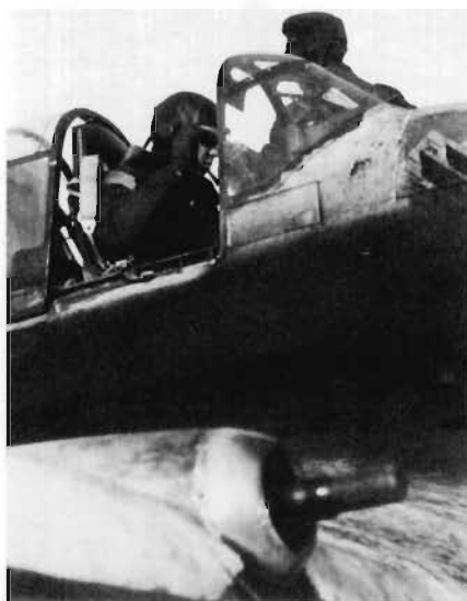
A close up of the short-barrelled Mauserwerk MG 181 in the wing of a Ju 87 D.
