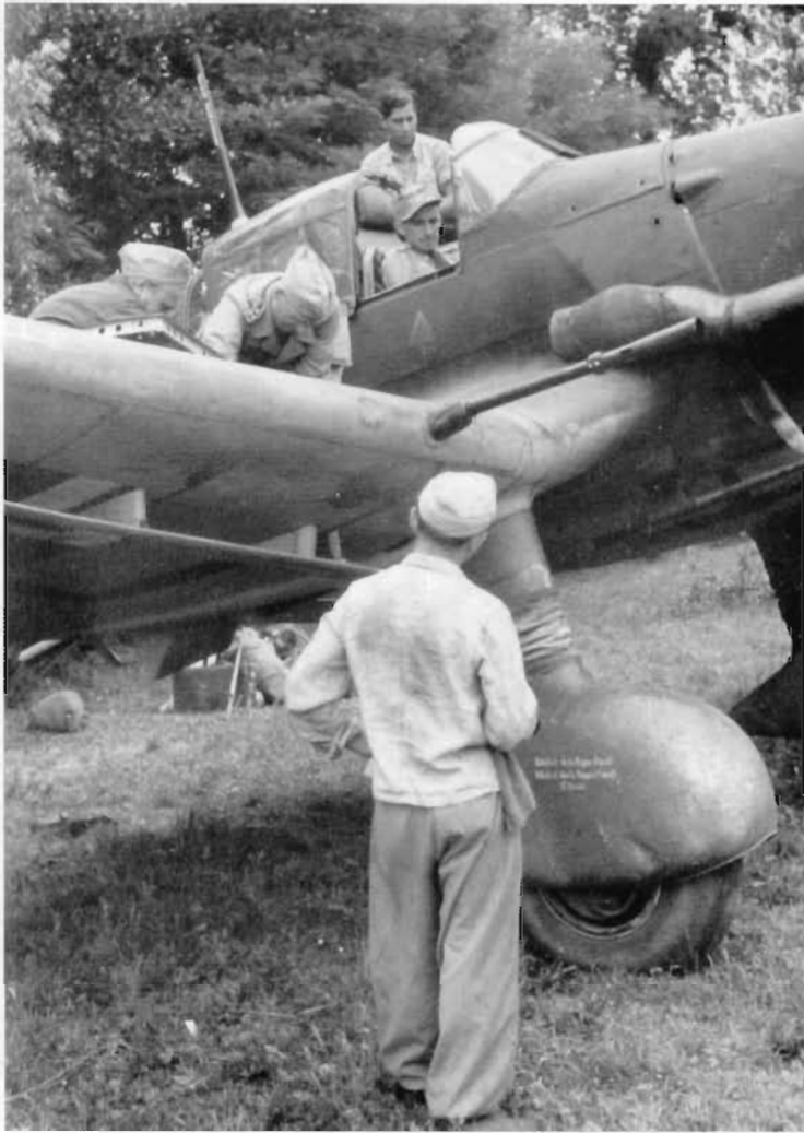
The flame dampers on this similarly camouflaged Ju 87 D-5 of NSG 9 have been extended to lead back over the wing leading edge, and flash suppressors have been added to the barrels of the MG 151 cannon.
