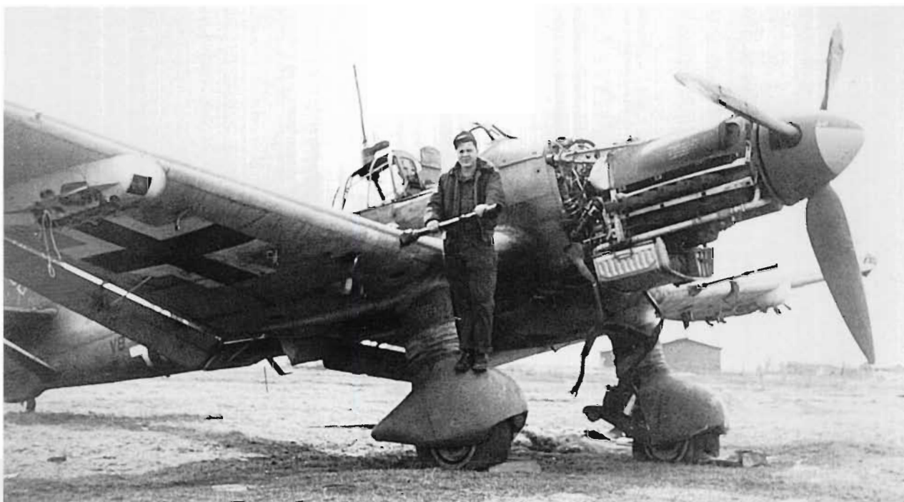
These photographs show a still remarkably intact Ju 87 D-5 coded V8+TD of NSG 1 (Süd) at Neubiberg in the autumn of 1946. Both wing-mounted MG 151 cannons have been fitted with flash suppressors and the fairing on the radio mast would normally have carried a loop aerial for the FuG 16.
