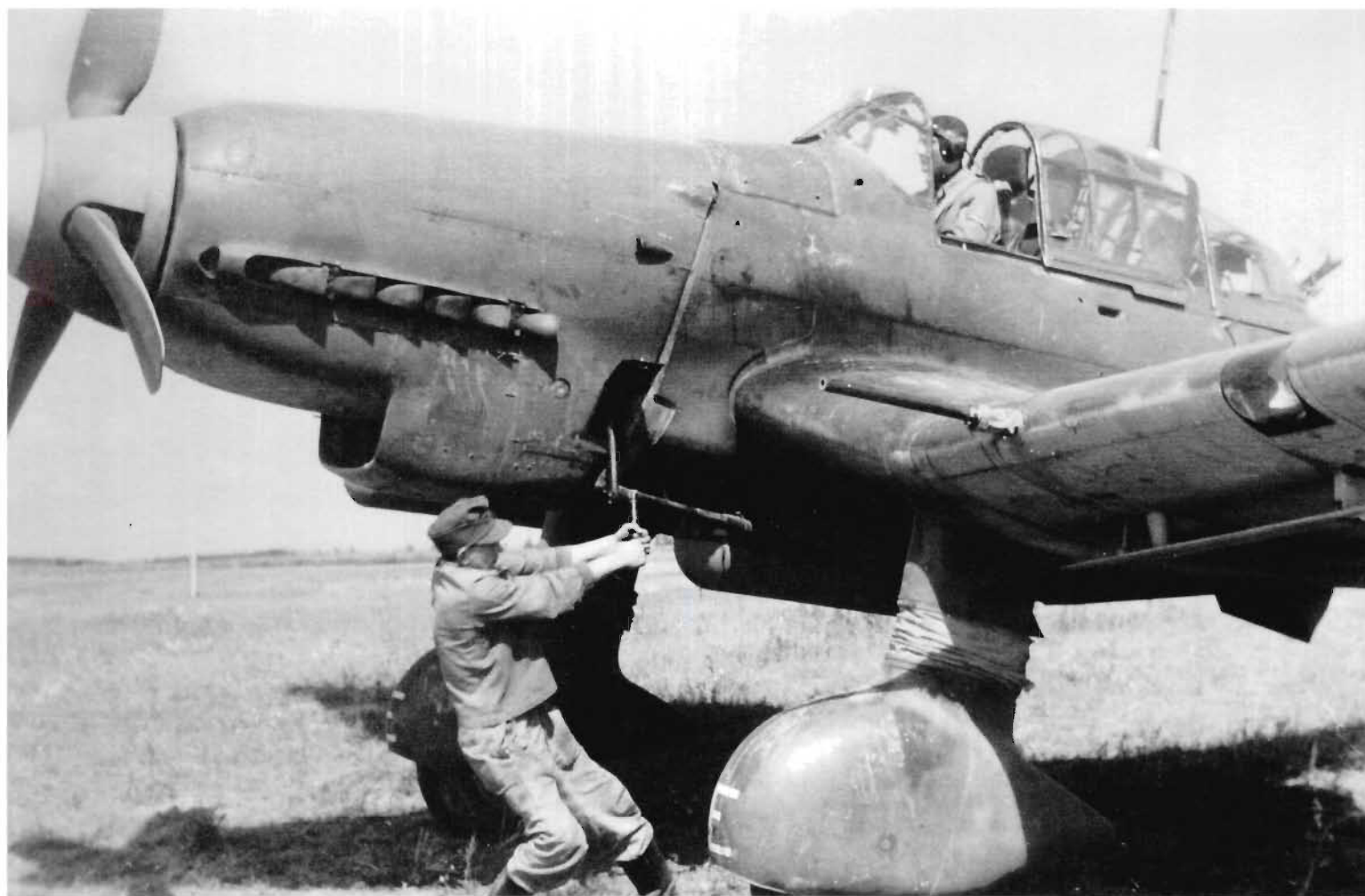
Two views of a Ju 87 D-5 preparing for a sortie on the Eastern Front, probably in the summer of 1944. Note the MG 151 cannon in the wings and the bulged Plexiglas fairing for the repositioned gun and bombsight above the windscreen. The D-5 also had the facility of jettisoning its undercarriage in an emergency by detonating explosive bolts which connected them to the main spar.
