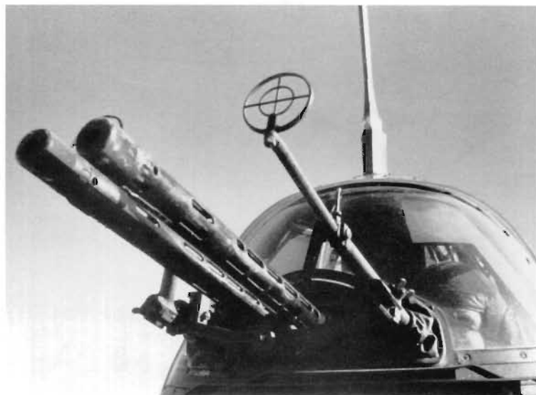
Another view of the twin rear firing MG 81Z machine guns, with the gunner peering through the uniquely shaped internal armour, known as the Gleitschienenlafette GSL-K 'citadel'. This was introduced in the Ju 87 D along with the reprofiled canopy.
