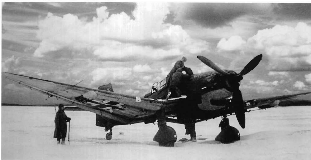
A Ju 87 D-5, aircraft letter B, captured by Soviet forces in the winter of 1944/45. Although missing, the spinner would almost certainly have been decorated with a white spiral, as shown (bottom) on a similar Ju 87 D from the same unit, but with the individual aircraft letter L. Although lacking flame dampers over the exhausts, the flash suppressors on the barrels of the MG 151 cannon suggest these aircraft belonged to a Nachtschlachtgruppe .
