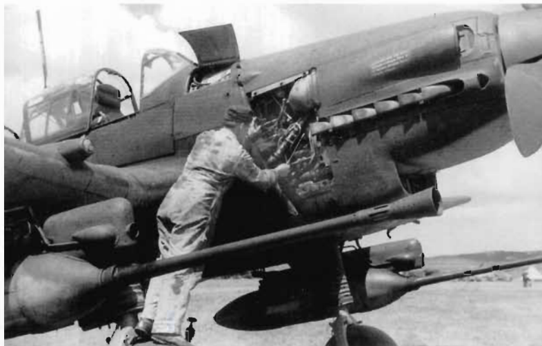
A groundcrew man carries out maintenance to the rear of the Jumo 211 F of a Ju 87 G.
