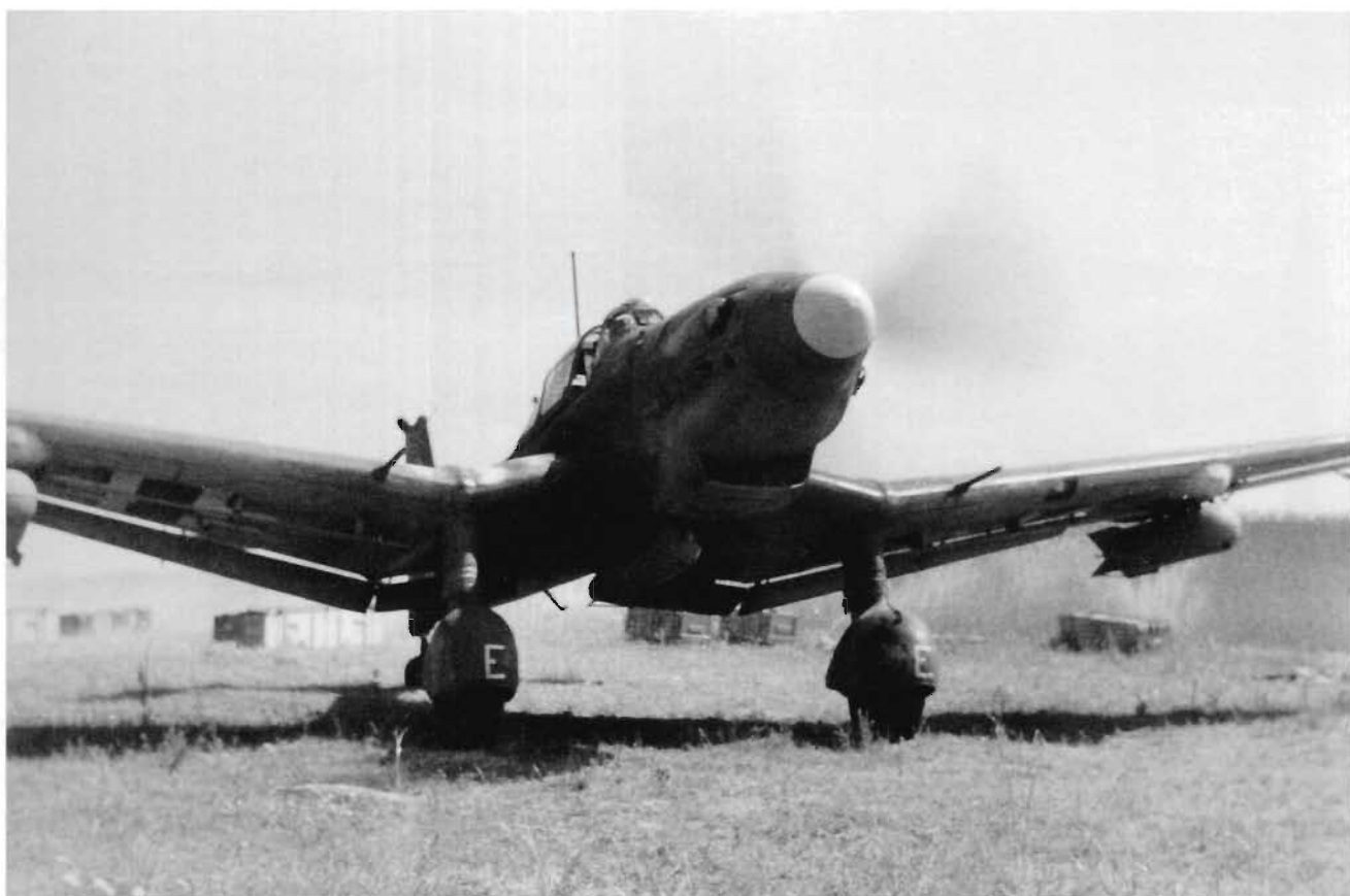
Two views of a Ju 87 D-5 preparing for a sortie on the Eastern Front, probably in the summer of 1944. Note the MG 151 cannon in the wings and the bulged Plexiglas fairing for the repositioned gun and bombsight above the windscreen. The D-5 also had the facility of jettisoning its undercarriage in an emergency by detonating explosive bolts which connected them to the main spar.
