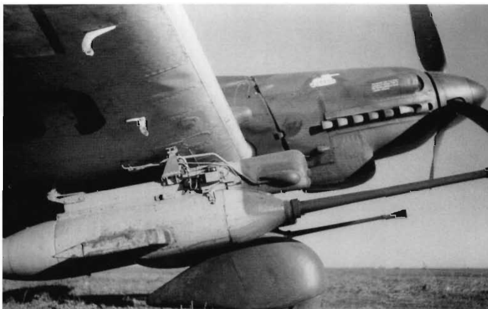
Two views of a Ju 87 G from St.G 1, marked with the T-34 Panzerknacker badge. The aircraft were often called Kannonenvogel (the "gun bird"). Thought devastating to Soviet armour these twin 37 mm cannon equipped Ju 87 Gs suffered a loss of speed and manoeuvrability due to the additional weight of the cannon at 700 kgs (350 kgs each).
