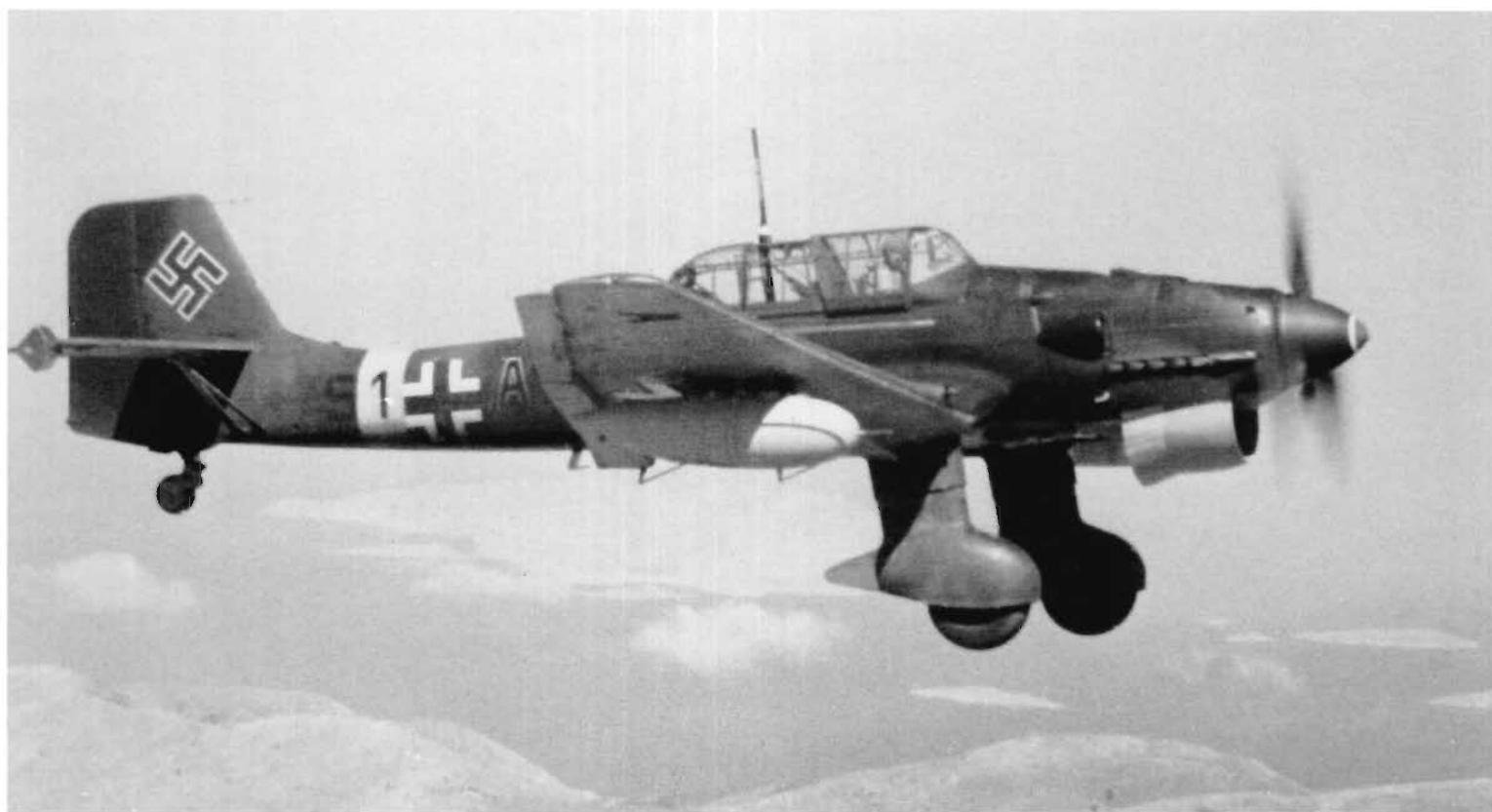
This Ju 87 R-2 coded S1+AM was flown by the Staffelführer of 4./St.G 3. The long range tanks and the lack of a gunner/wireless operator suggests the machine was on a ferry flight when photographed.
