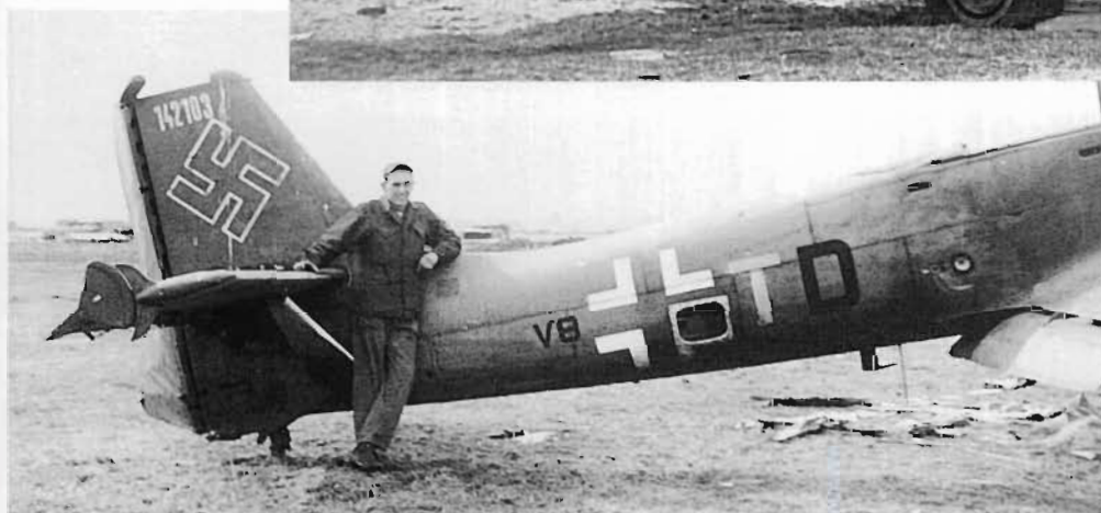
These photographs show a still remarkably intact Ju 87 D-5 coded V8+TD of NSG 1 (Süd) at Neubiberg in the autumn of 1946. Both wing-mounted MG 151 cannons have been fitted with flash suppressors and the fairing on the radio mast would normally have carried a loop aerial for the FuG 16.
