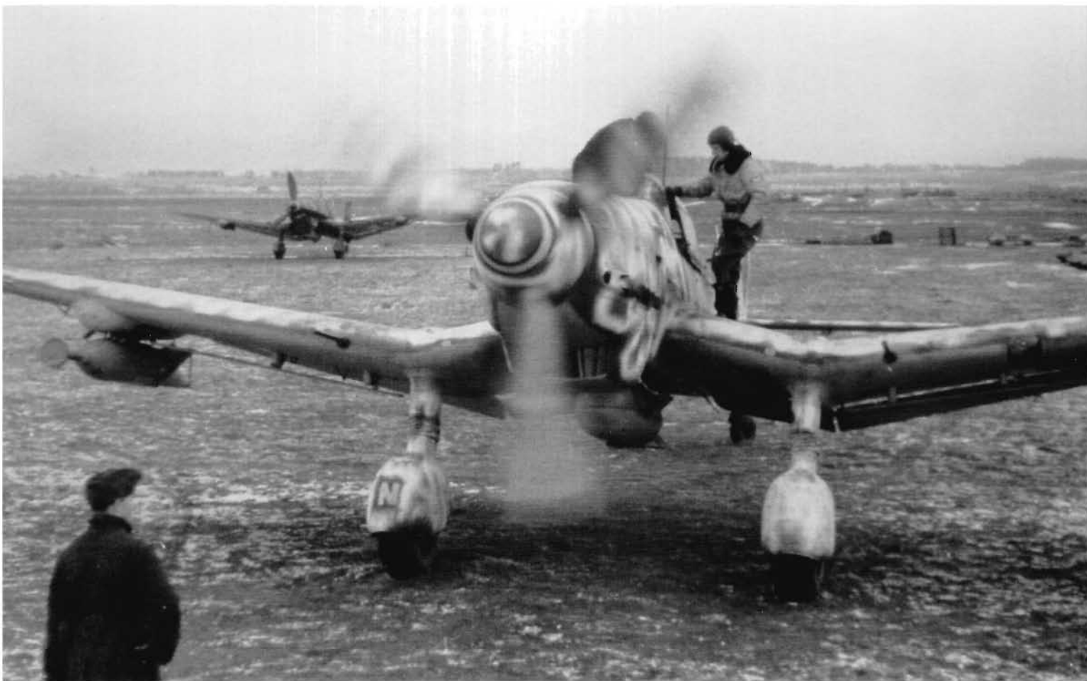
Above and opposite page: Another variation of the winter scheme is seen on a Ju 87 D-5, believed to be a machine of SG 2, in the winter of 1943/44. The camouflage has been applied with the aid of a spraygun in a white meander pattern which also included the spinner and propeller blades. The aircraft is armed with SD 250 bombs fitted with extended fuses under the wings and an AB 500 container under the fuselage.
