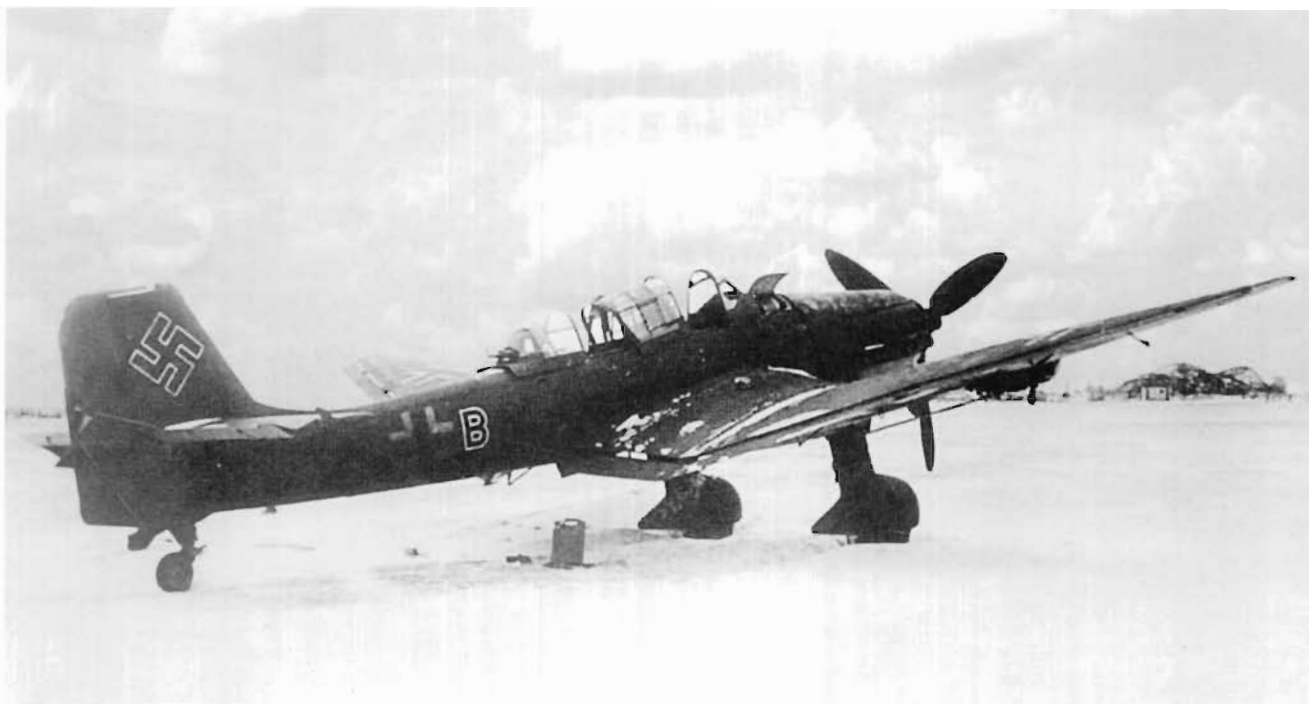
A Ju 87 D-5, aircraft letter B, captured by Soviet forces in the winter of 1944/45. Although missing, the spinner would almost certainly have been decorated with a white spiral, as shown (bottom) on a similar Ju 87 D from the same unit, but with the individual aircraft letter L. Although lacking flame dampers over the exhausts, the flash suppressors on the barrels of the MG 151 cannon suggest these aircraft belonged to a Nachtschlachtgruppe .
