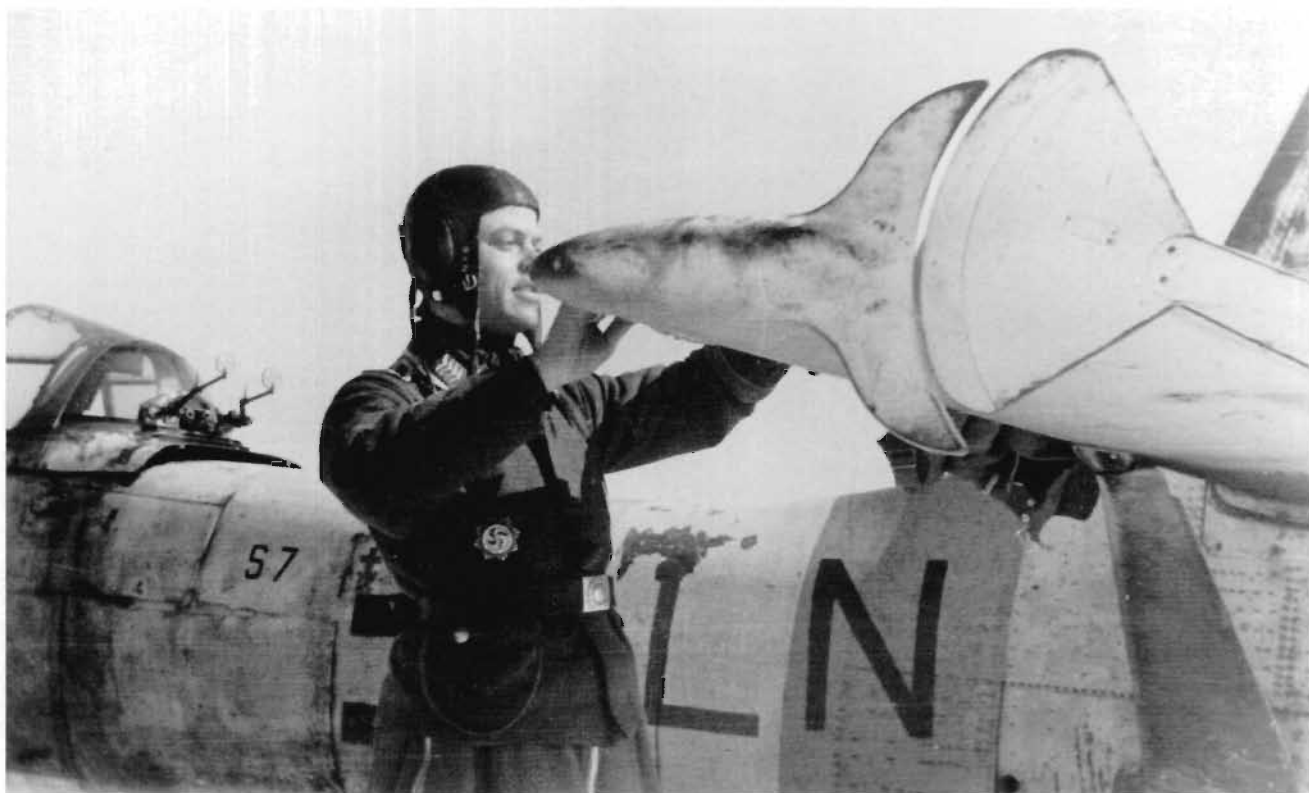
Above and opposite page: Another variation of the winter scheme is seen on a Ju 87 D-5, believed to be a machine of SG 2, in the winter of 1943/44. The camouflage has been applied with the aid of a spraygun in a white meander pattern which also included the spinner and propeller blades. The aircraft is armed with SD 250 bombs fitted with extended fuses under the wings and an AB 500 container under the fuselage.
