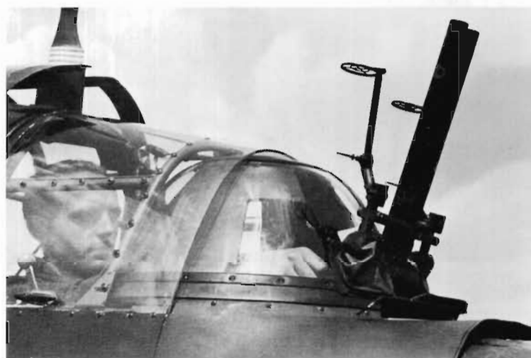
A close up of the twin rear firing MG 81Z machine guns in the rear cockpit of a Ju 87 D.
