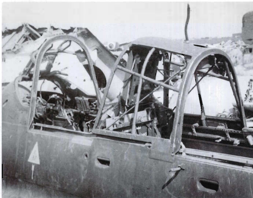
The remains of a night ground attack Ju 87 D-3 at Prague - Rusin in 1945. Note that most of the canopy framing on all variants of the Ju 87 was under the Plexiglas.
