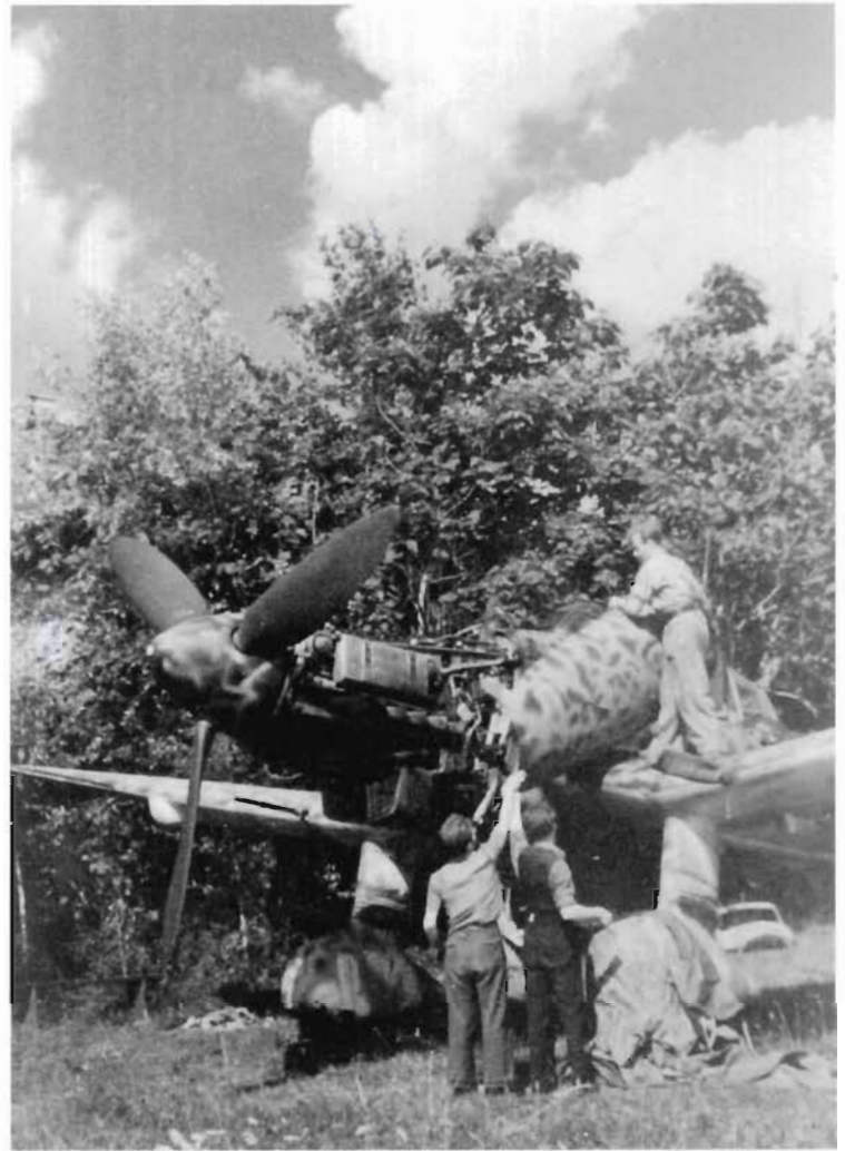
Ground crew replacing the cowlings on a Ju 87 D of NSG 9 in Italy.
