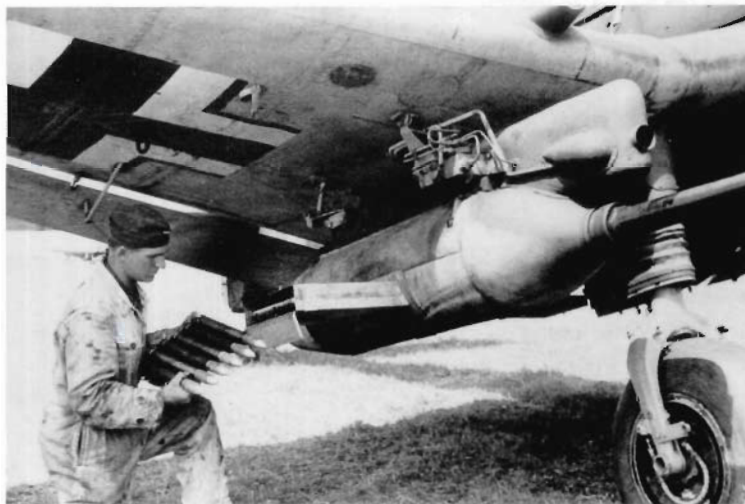
Two views of a Luftwaffe armourers about to load a clip of 37 mm anti-tank rounds into the magazine holder of a BK 3.7 cannon.
