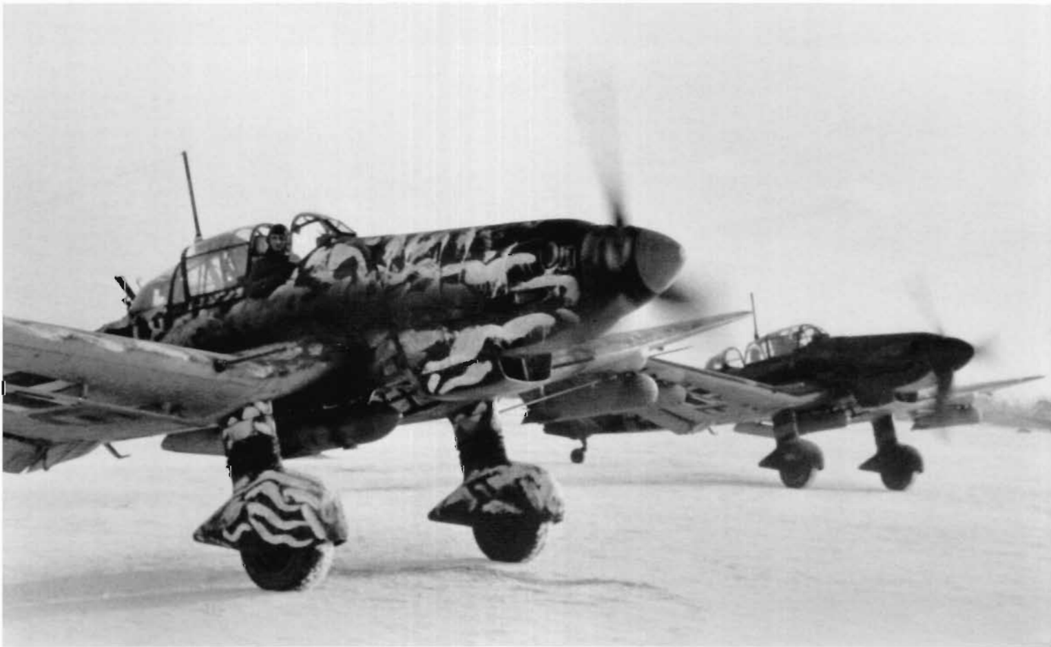
A particularly untidy snow scheme, evidently applied by brush in the winter of 1943/44. The aircraft, a Ju 87 D-5, is armed with AB 250 bomb containers on the wing racks. The Soviets named these cluster weapons 'Frogs' because of the noise they made when heard exploding in the distance.
